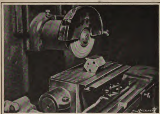
Fig. 4. Grinding One Side of Thread-cutting Tool on Surface Grinder
